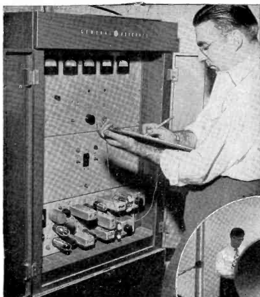
S-T Link —transmitter shown here—feeds programs from master studio in Ithaca to broadcast transmitter on hilltop—a distance of 9.5 miles. Microwave “dish” antennas (right) are mounted on studio building and on transmitter house.
